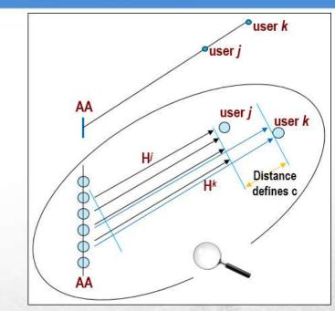
If two users **j** and **k** are located on the same beam then their channel vectors are close to collinear
